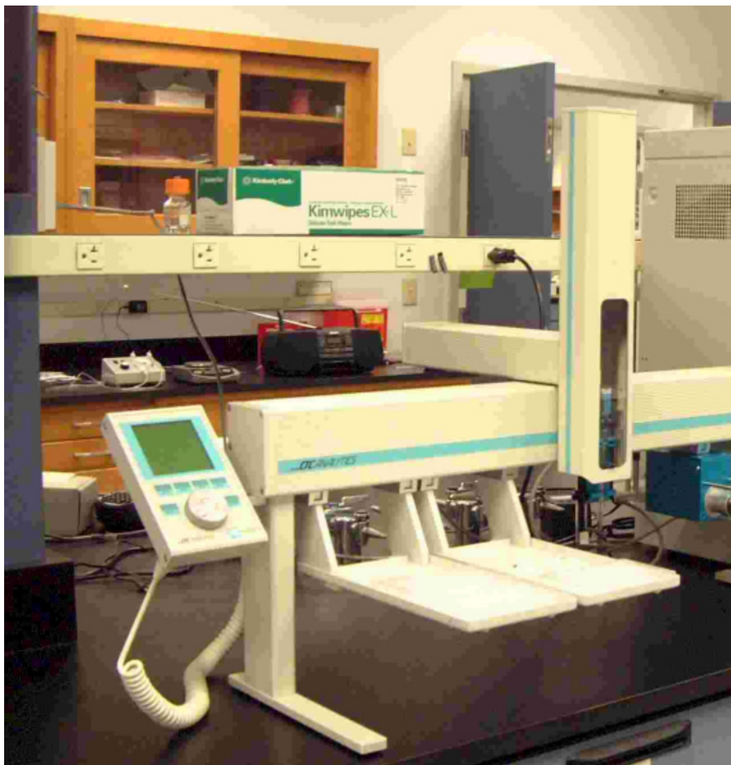
Figure 1. Protasis MicroFlow NMR Automation system consisting of Protasis CapNMR probe, a CTC/Leap Technologies capillary-scale LC PAL liquid handler, Protasis Discovery Tower fluidic platform, and Protasis OneMinuteNMR
